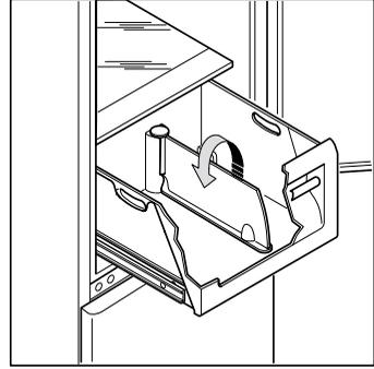
To remove the drawer, use the side handles (as shown in the drawing). All parts inside the drawer can be removed for cleaning purposes.
