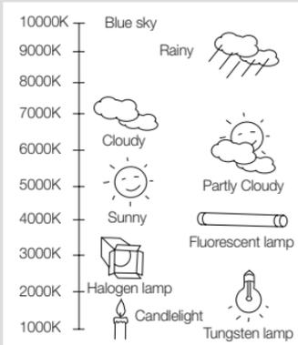
※1 : With <ATW1> mode active in a color temperature environment ranging beyond between 2500K and 9300K, a proper white balance value may not be produced; if this is the case, you are recommended to use <ATW2> mode.
