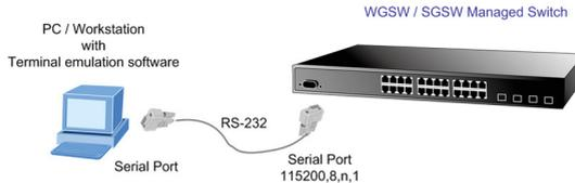
A terminal program is required to make the software connection to the WGSW / SGSW Managed Switch. Windows' Hyper Terminal program may be a good choice. The Hyper Terminal can be accessed from the Start menu.
