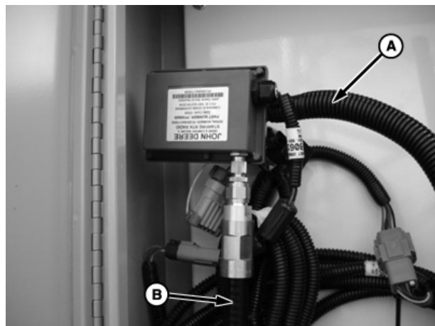
A —91.4 m (300 ft) RS232 Cable from receiver
