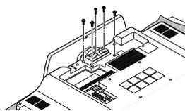
2) Tighten the 5 screws to the back of the TV.
