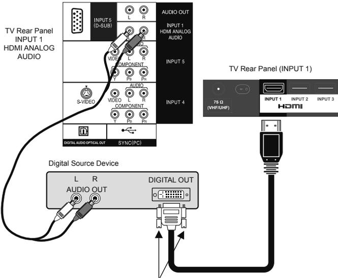
After the connections have been made, tighten the screw to secure the cables.
