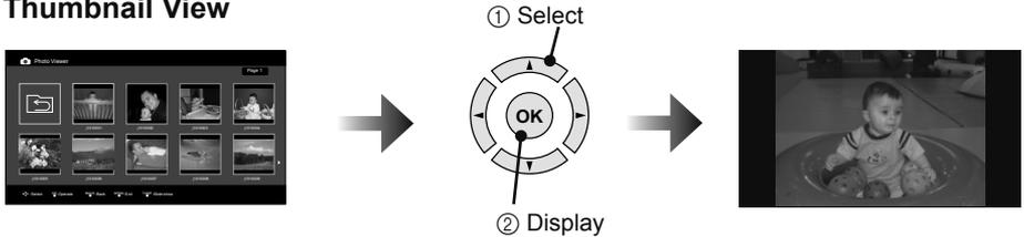
When you select **Thumbnail view** and press **OK**, a folder or file list will be displayed. Select your folder by using the ◀▶ or ▲▼ buttons. Choose a picture and press the **OK** button. It will now be shown on the screen. To move to the next picture, press the ▶ button. To move to the previous picture, press the ◀ button.
