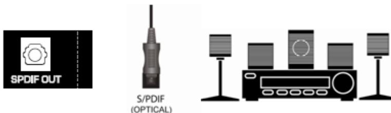
If your sound system has a S/PDIF (optical) digital audio input you can connect it from your sound system to the **OPTICAL** digital audio out on your HDTV. This is active when receiving audio with the programs being viewed no matter what input is being used.
