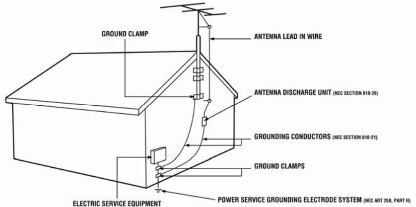
**Remember, the screen of the coaxial cable is intended to be connected to earth in the building installation.**
