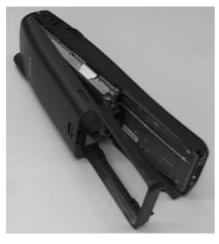
3. The back lower case assy and battery plate can now be separated from the upper case.
