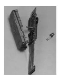
8. When the spring is taken off, the RF/Logic unit can be lifted. The centre bolt (MMI support) can now also be taken away. Note that the centre bolt is not symmetric (comparing both ends). The shorter end fits into the MMI board.
