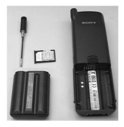
1. Remove Simcard holder, antenna (no tool needed), battery cover and battery.
