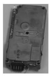
10. The RF/Logic unit is 1 item, it should never be disassembled. Separate parts are not available. The IMEI number in the RF/Logic memory has to be equal to the IMEI number on the battery plate assy.
