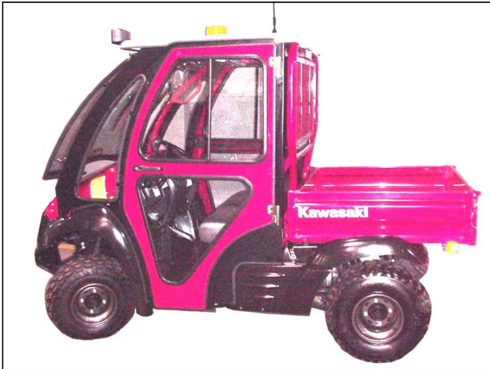
This cab is shown with the following optional equipment: hard sided doors, work lights, windshield wiper, strobe light, and antenna for overhead console. Other options not shown are: soft sided doors and an anti-draft panel for underneath the bench seat.
