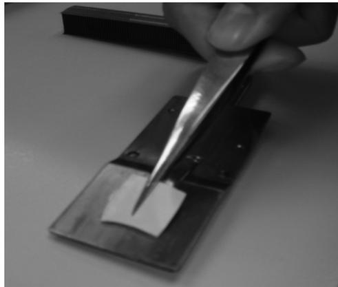
*Figure 4-20 Replace new thermal pad into correct position.*
