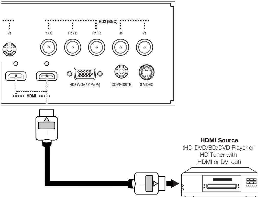
**Figure 3-11. HDMI Source Connections**
