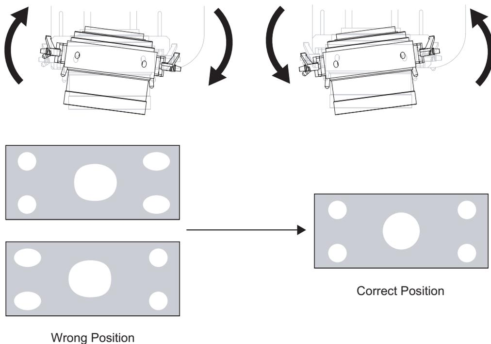
Once the proper lens angle has been set, firmly tighten the Yaw/X-Adjustment Levers to secure the lens in place.
