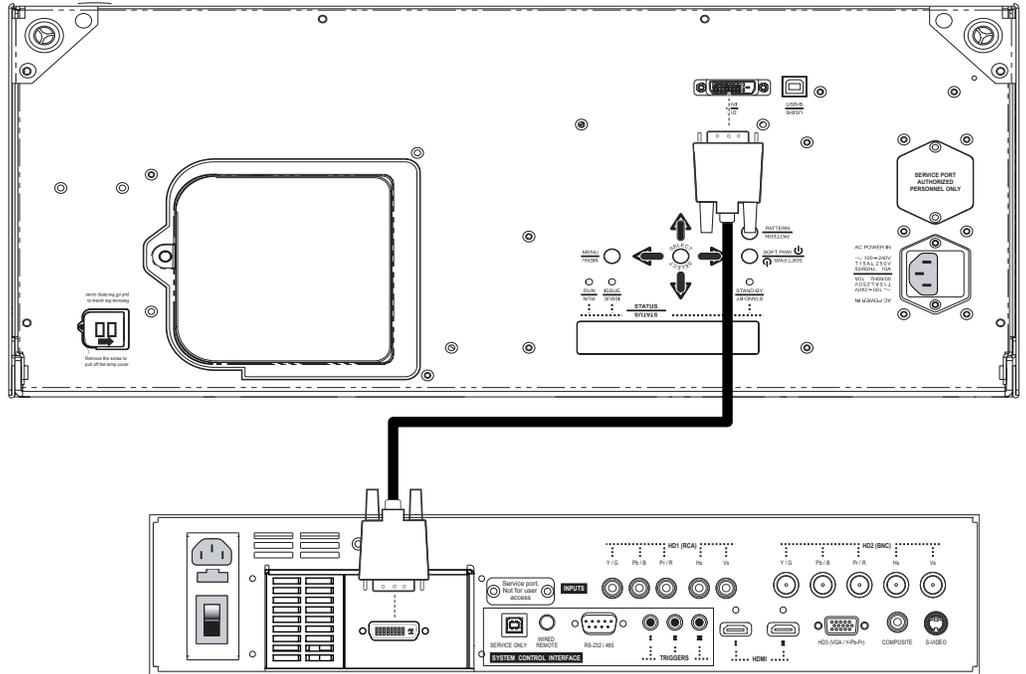
**Figure 3-10. Connecting the VX-33d to the DHD Controller**
