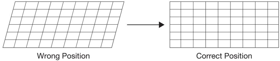
4. When the image geometry appears correct, tighten the Anamorphic Lens Set Screw (item #10) to secure the lens in place. (When viewed from the front, the rear opening on the anamorphic lens should appear as a tall, narrow oval.)
