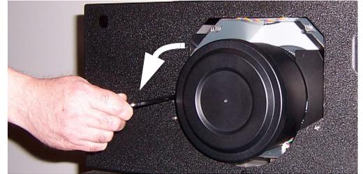
8. Replace the Lens Cavity Front Cover.
