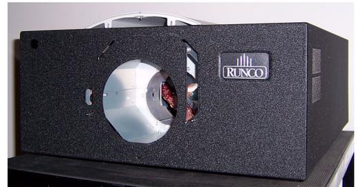
3. Remove the Lens Cavity Front Cover.
