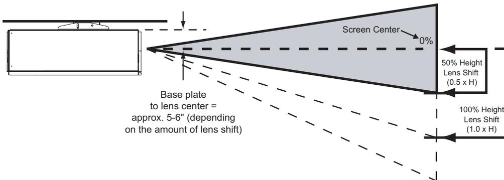
**Note:** This is a general example of lens shift. Lenses vary in their shift capabilities. **No particular lens or projector is used in this example.**
