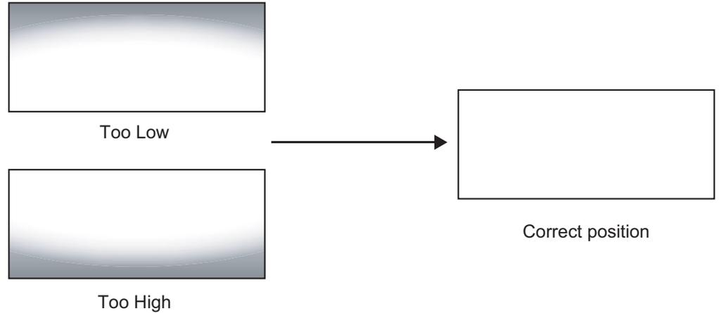
When the height is properly set, tighten the Height Adjustment T-Screws to secure the lens in place.
