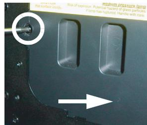
3. Slide the Lamp Cover in the direction of the arrow to remove it.
