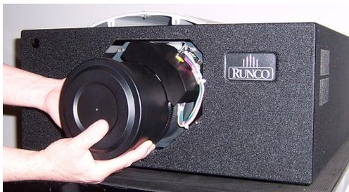
6. Carefully rotate the lens assembly 45 degrees clockwise until the motor socket connector is aligned with the connector on the flange. Then, gently push the lens assembly in until it is seated flush against the flange and the connectors have seated.
