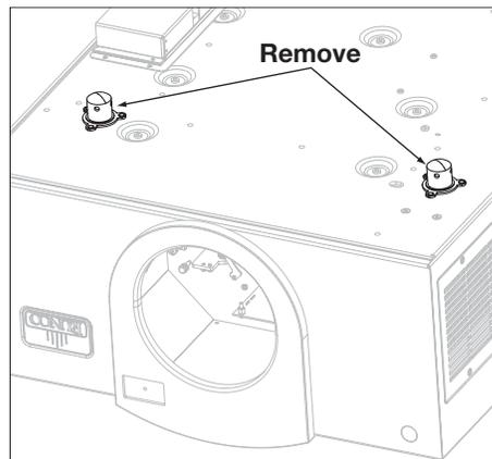
**Install Ceiling Mount Adapters/Projector Stands:** For ceiling installations, the adapters bring the attachment points for the projector mounting rails (included with the projector ceiling mount kit) from the bottom of the projector up and around the AutoScope lens motor housing. For floor installations (where the projector is upright), the adapters allow the projector to lie flat on the mounting surface.
