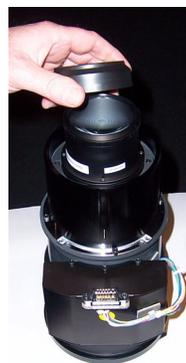
5. Hold the lens assembly with the motor facing the upper-right corner of the Lens Cavity. **Carefully** insert the back of the lens assembly into the hole in the lens flange.
