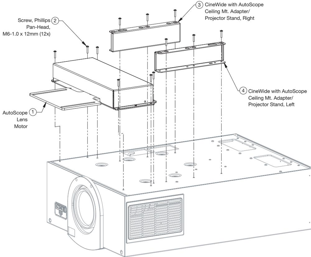
**Figure 3-6. VX-33d/CineWide with AutoScope Motor Assembly - Exploded View**
