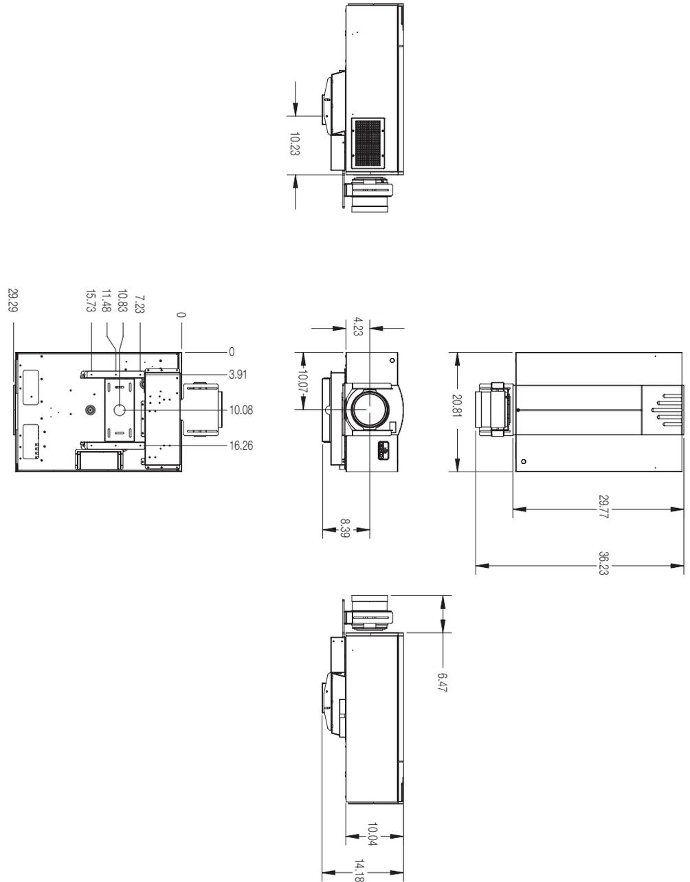
**Figure 7-1. VX-33d Dimensions (with Ceiling Mount and CineWide/AutoScope Options)**
