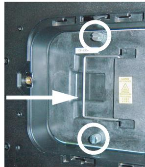
5. Grasp the lamp assembly handle and pull gently, removing the lamp module from the projector housing.
