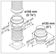
In some cases, a condensate trap may also be required to collect and evaporate any condensate which may occur. This optional accessory is available for ducts 5" (125 mm) and  $5^{7}/8$ " (150 mm) in diameter.
