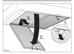
■ To remove the grease filters pull the locking clips, 1, forward. Lower the filter 45°, 2, unhook it at the rear, 3, and take it out. Support the grease filter so that it does not fall onto the cooktop.
