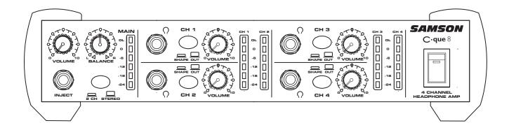
MASTER VOLUME – Off ST/2CH SWITCH – Out MASTER BALANCE- Center, 12:00 CHANNEL 1 VOLUME – 0
