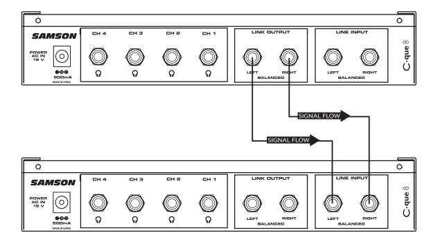
Because the C•que 8 Stereo Link output jacks are electronically balanced, we recommend the use of 3-conductor cable and 1/4" TRS (Tip/Ring/Sleeve) connectors. Even when several C•que 8's are linked together this way, there is no loss of power or audio fidelity—every Channel on every C•que 8 will sound just as loud and clear as if it were the only unit connected. The status of the front-panel Stereo/2 CH buttons affects only that unit and has no effect on any subsequent linked units.
