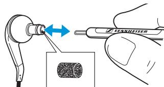
► Replace dirty diaphragm guards using the cleaning tool or tweezers.
