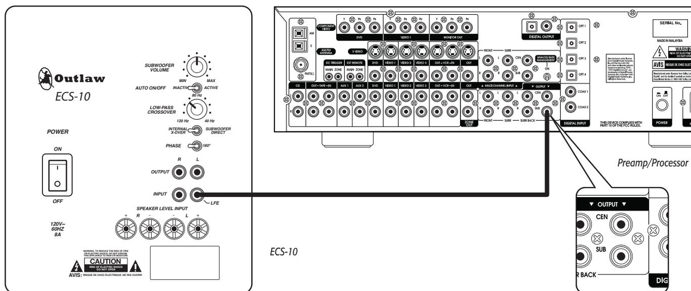
**Diagram 2: Connecting to a System without a Subwoofer Preamp Output, but with Standard Left/Right Preamp Outputs**
