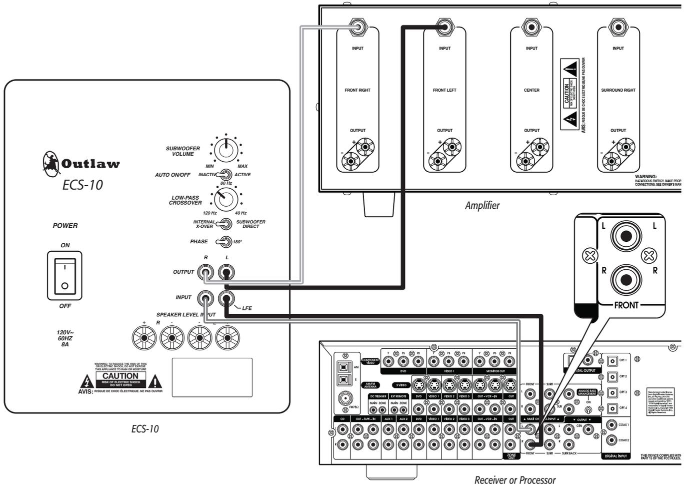
5. Plug the ECS-10's power cord into an un-switched AC outlet.
