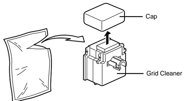
**NOTE:** The pad of the grid cleaner contains water. Clean the grid quickly so that the pad may not dry off.
