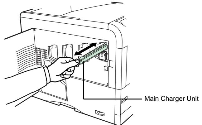
**NOTE:** If the main charger unit is not restored to its home position, the corresponding color will be printed over the whole page.
