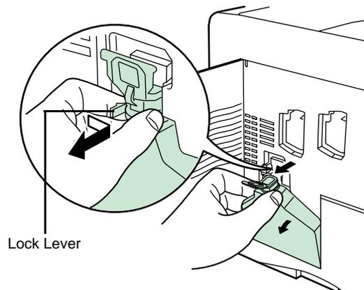
**NOTE:** Remove the waste toner box as gently as possible so as not to scatter the toner inside. Do not let the opening of the waste toner box face downward.
