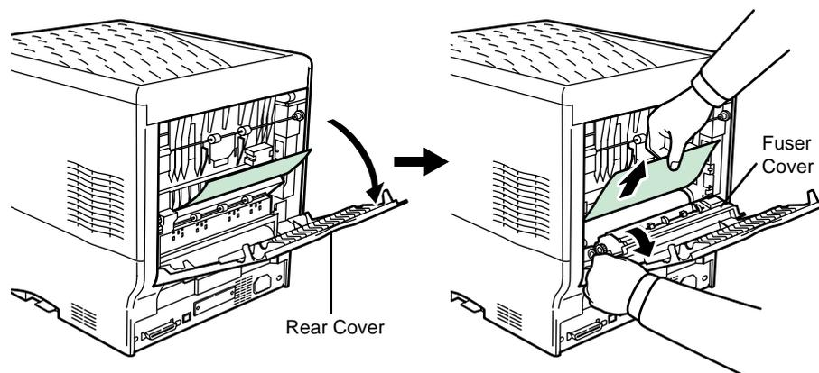
**CAUTION:** The fuser unit inside the printer is hot. Do not touch it with your hands as it may result in burn injury. Remove jammed paper carefully.
