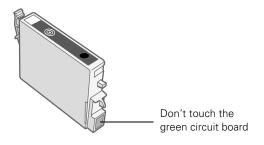
7. Lower the cartridge into the holder, with the green circuit board facing the front. Then gently push the cartridge down until it clicks into place.
