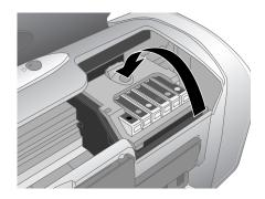
10. Close the printer cover and press the ◊ ink button. The printer begins charging the ink delivery system.
