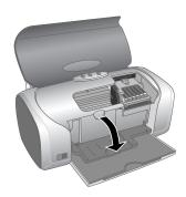
3. Place the CD or DVD on the CD/DVD tray with the white or printable side face-up. Make sure the disc lays flat in the tray.
