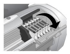
5. Press in the tab on the back of the cartridge and lift the cartridge out of the printer. Dispose of it carefully.
