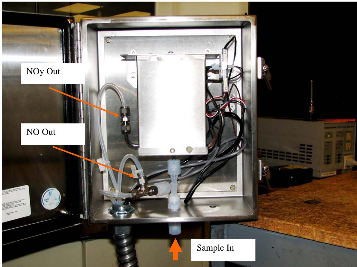
**Figure 5.2 - Converter Assembly**
