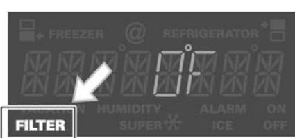
The age of the filter is close to the maximum life time. Order a new "UltraClarity" water filter.
