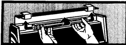
2. Remove lamp socket safety cover at each end of the fluorescent tube.
