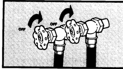
**WHEN NOT WASHING,** keep both water faucets turned off. This takes the pressure off the water inlet valve and hoses.
