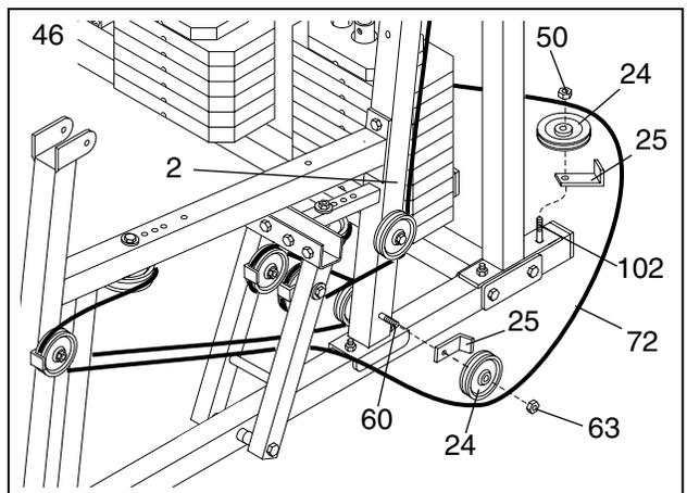
47. Route the threaded end of the Press Cable (72) around the 3 1/2" Pulley (24) that was mounted on the bracket on the Weight Base (5) in an earlier step.
