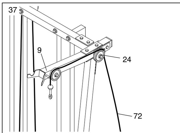
38. Wrap the Press Cable (72) around a 3 1/2" Pulley (24) in the direction shown. Attach the Pulley to the indicated hole in the Press Upright (2) with a 3/8" x 3 3/4" Bolt (59), a 3/8" Flat Washer (48) and a 3/8" Nylon Locknut (50). **Make sure the Cable Trap is oriented as shown.**
