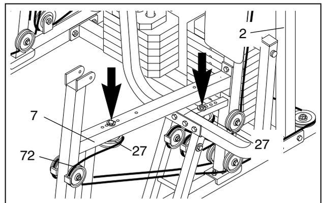
The threaded ends on the Press Cable (72) and the Ab Cable (74) that are attached to the weight stacks can also be used to tighten the cables.
