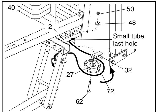
41. Route the Press Cable (72) back through the opening in the Press Frame (8) and wrap the Press Cable around a 3 1/2" Pulley (24) in the direction shown. Then, route the Press Cable back through the opening in the Press Frame (8).
