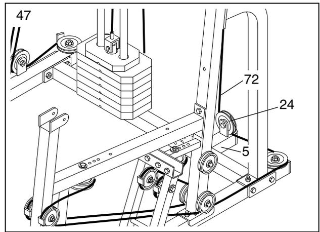
48. Wrap the Press Cable (72) over a 4 1/2" Pulley (82) in the direction shown. Attach the Pulley inside the indicated bracket on the Weight Top Frame (66) with a 3/8" x 1 3/4" Bolt (57) and a 3/8" Nylon Locknut (50). **Make sure the end of the Cable is routed through the bracket, as shown.**
