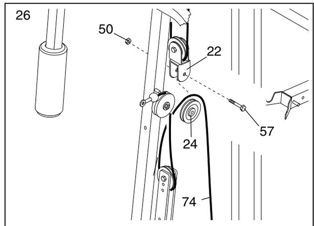
27. Wrap the Ab Cable (74) around a 3 1/2" Pulley (24) in the direction shown. Attach the Pulley and a Cable Trap (25) to the welded bracket on the Butterfly Base (4) with a 3/8" x 2" Bolt (54) and a 3/8" Nylon Locknut (50). **Make sure the Cable Trap is oriented as shown.**
