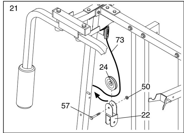
22. Wrap the Butterfly Cable (73) around a "V"-Pulley (27) in the direction shown. Attach the "V"-Pulley and a Large Cable Trap (32) to the bracket **on the back of the Butterfly Upright (1)** with a 3/8" x 2 1/2" Bolt (53) and a 3/8" Nylon Locknut (50). **Make sure the Large Cable Trap is oriented as shown.**
