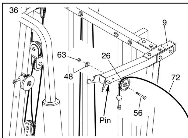
37. Route the threaded end of the Press Cable (72) around the 3 1/2" Pulley (24) that is already mounted on the Top Frame (9).
