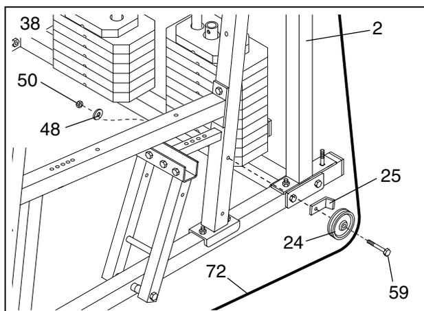
39. **Important: Although the following steps are not difficult to perform, the correct routing of the cable is critical to the functioning of the home gym. Please make sure that you wrap the cable around the pulleys exactly as shown in each step.**
