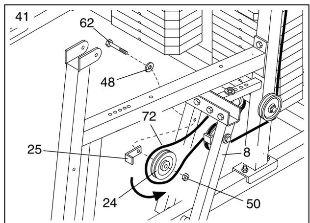
42. Wrap the Press Cable (72) around a 3 1/2" Pulley (24) in the direction shown. Attach the Pulley and a Cable Trap (25) to the indicated hole **on the far side of the Press Upright (2)** with a 3/8" x 4 3/4" Bolt (60) and a 3/8" Nylon Jamnut (63). **Note: Thread the Jamnut only two turns onto the Bolt; you will later attach another Pulley to the Bolt. Make sure the Cable Trap is oriented as shown.**
