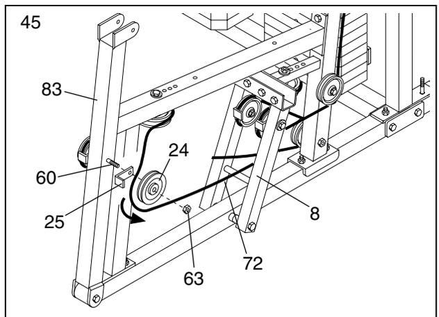
46. Wrap the Press Cable (72) around a 3 1/2" Pulley (24) in the direction shown. Attach the Pulley and a Cable Trap (25) to **near side** of the Press Upright (2). Use the 3/8" x 4 3/4" Bolt (60) that was inserted in step 42 and secure the Pulley with the 3/8" Nylon Jamnut (63). **Make sure the Cable Trap is oriented as shown.**
