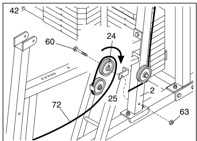
43. Wrap the Press Cable (72) around a 3 1/2" Pulley (24) in the direction shown. Attach the Pulley and a Cable Trap (25) to the indicated hole **on the far side** of the Leg Press Lever (83) with a 3/8" x 4 3/4" Bolt (60) and a 3/8" Nylon Jamnut (63). **Note: Thread the Jamnut only two turns onto the Bolt; you will later attach another Pulley to the Bolt. Make sure the Cable Trap is oriented as shown.**
