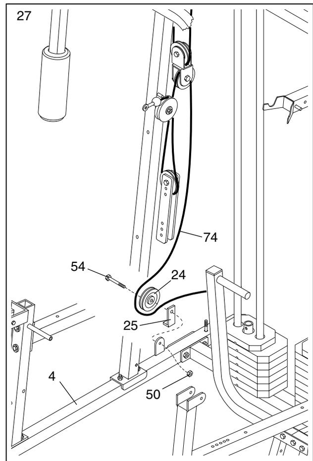
28. Wrap the Ab Cable (74) around a 3 1/2" Pulley (24) in the direction shown. Slide the Pulley and a Cable Trap (25) onto the 3/8" x 3 1/2" Carriage Bolt (95) already inserted into the Butterfly Base (4). Secure the Pulley with a 3/8" Nylon Jamnut (63). **Make sure the Cable Trap is oriented as shown.**
