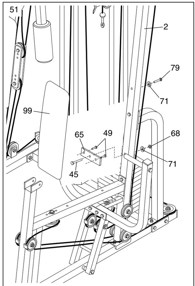
52. Insert a 1/4" x 2 1/2" Carriage Bolt (45) through the center hole in a Seat Plate (65). Attach the Seat Plate to a Seat (13) with two 1/4" x 3/4" Bolts (49).
