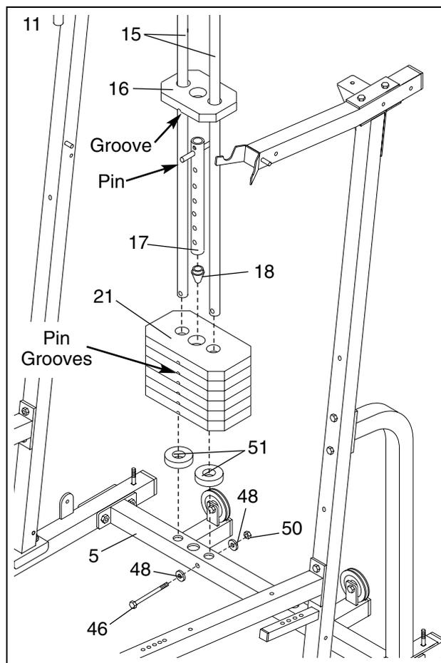
12. Place two Weight Bumpers (51) over the indicated holes in the Weight Base (5). Slide a Weight Guide (15) into each of the holes.
