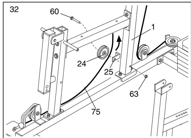
33. Wrap the Low Pulley Cable (75) over a 3 1/2" Pulley (24) in the direction shown. Attach the Pulley and a Cable Trap (25) to the lower hole in the Adjustable Pulley Plates (23) with a 3/8" x 2" Bolt (54) and a 3/8" Nylon Locknut (50). **Make sure the Cable Trap is oriented as shown.**
