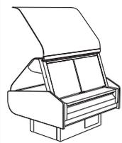
**Hood glass extended to the full, upright portion is stabilized through the use of gas struts designed for the full, load-bearing weight. These struts could weaken or fail due to wear, environmental conditions or aging. OPERATORS SHOULD BE AWARE OF ANY DECREASE IN EFFORT TO LIFT THE HOOD AND INITIATE AN IMMEDIATE GAS STRUT SAFETY CHECK. DO NOT LIFT THE HOOD IN THIS CONDITION.**
