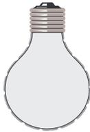
The performance of this unit has been optimized using the factory provided bulbs. These bulbs should be replaced with an exact replacement or with a factory recommended replacement. These bulbs have been treated to resist breakage and must be replaced with similarly treated bulbs in order to maintain compliance with NSF standards. **DO NOT** over-tighten bulbs in their receptacles as this can cause damage to the bulb filament.
