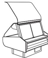
Hood glass extended to the full, upright portion is stabilized through the use of gas struts designed for the full, load-bearing weight. These struts could weaken or fail due to wear, environmental conditions or aging. OPERATORS SHOULD BE AWARE OF ANY DECREASE IN EFFORT TO LIFT THE HOOD AND INITIATE AN IMMEDIATE GAS STRUT SAFETY CHECK. **DO NOT LIFT THE HOOD IN THIS CONDITION.**
