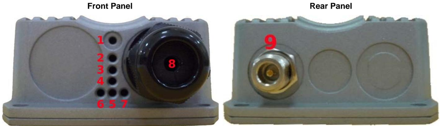
1. Reset Button : System reboot button press until LED flashed and release for system reboot or for reset to factory default press, LED flashes keep pressing until LED becomes static
