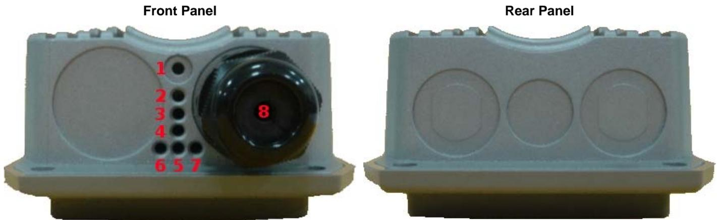
1. Reset Button : System reboot button press until LED flashed and release for system reboot or for reset to factory default press, LED flashes keep pressing until LED becomes static
