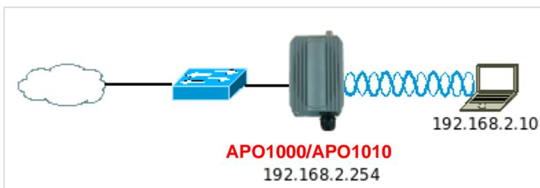
**Figure 3-1** Access Point on a Wired LAN Configuration
