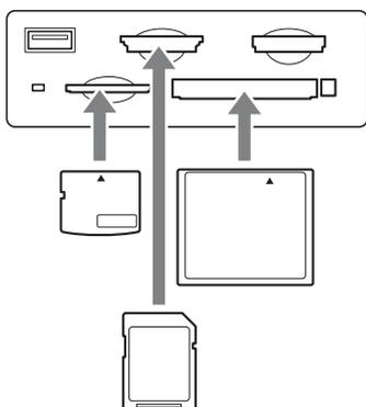
With the label facing up, fully insert the card in the direction indicated by ▲.
