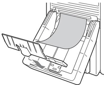
The output tray adapter prevents printouts from sticking out of the output tray. Use the adapter when printouts curl as shown.
