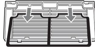
**3** Wash the filter with water to remove the dust.
