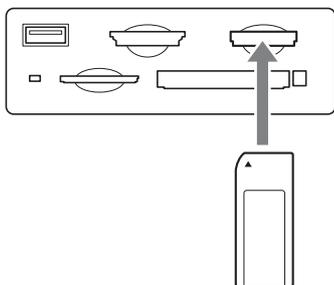
With the label facing up, fully insert the “Memory Stick” in the direction indicated by ▲.
