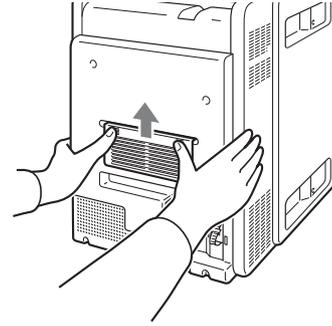
**2** Remove the filter from the filter cover.
