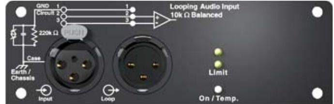
Figure 3.1. Side panel audio input connectors
