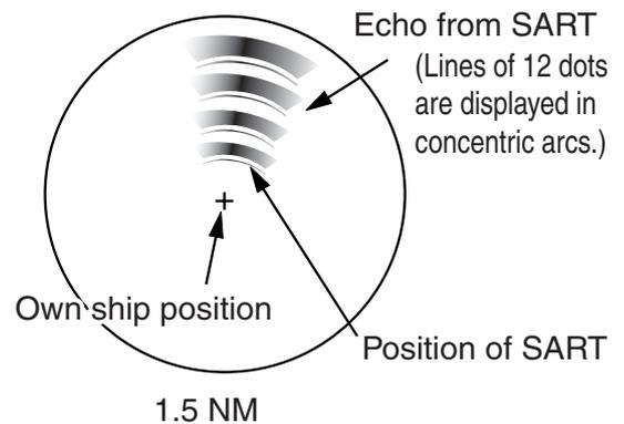
*Appearance of SART signal on the radar display***General procedure for detecting SART response**
