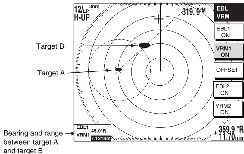
*Measuring range and bearing between two targets*
