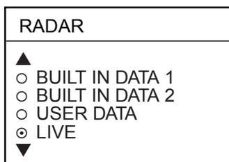
2. Select BUILT IN DATA 1 or 2 for internally generated echoes or USER DATA for user-saved radar data. Push the **ENTER** knob.
