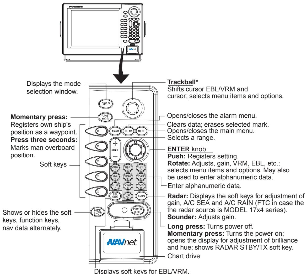
\*: When it has been some time since the trackball was last operated, the cursor may not track the movement of the trackball. In this case, move the trackball rapidly and then finely.
