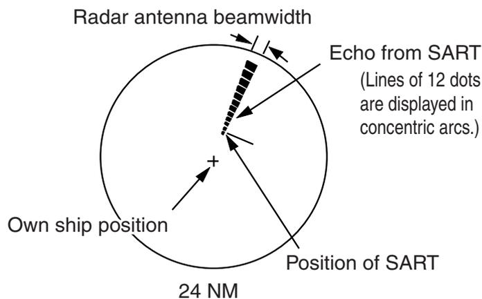
**Screen B: When SART is close**
