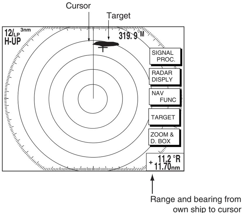
*How to measure range to a target with the cursor*
