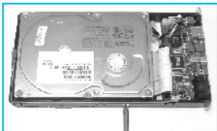
3. Re-insert the chassis into the enclosure.
