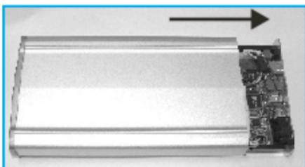
2. Connect the 40-pin IDE cable and 12 V power cable to the HDD. Fix in place with the included screws.
