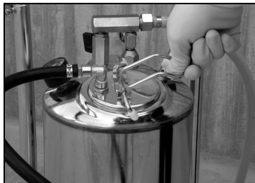
Flip over fastener and press down as far as it will go Insert pressure vessel in unit Secure bracket Connect air hose
