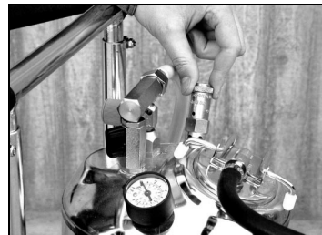
Close safety valve
