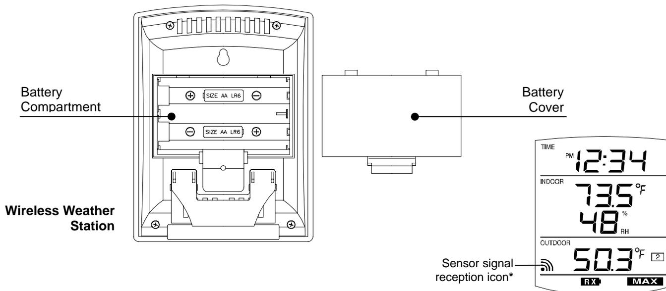
\* When the signal is successfully received by the Weather Station, the icon will be switched on. (If not successful, the icon will not be shown in LCD) So the user can easily see whether the last reception was successful (icon on) or not (icon off). On the other hand, the short blinking of the icon shows that a reception is being done now.
