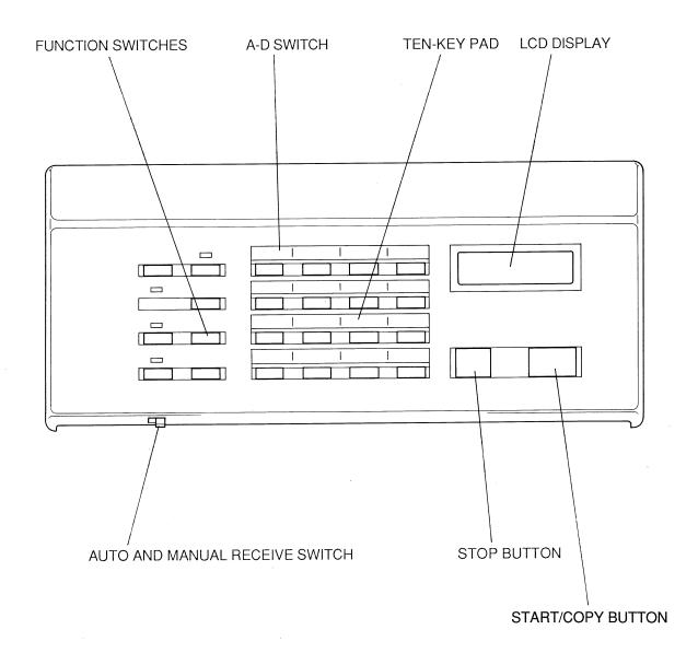
The proper utilization of the various buttons will be explained when we will describe the various operating modes of the FAX-1000.
