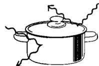
**Microwaves are absorbed by water, oil and fat.** The water, oil and fat molecules are excited by microwaves and rub against each other, just like when you rub your hands quickly against each other and heat is produced. The speed of rubbing determines the temperature. Microwave energy is not hot. It simply causes the food to make its own heat.
