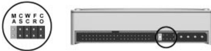
**Figure 7-13.** 2.1-GB Maxtor EIDE Hard Drive Jumper Settings
