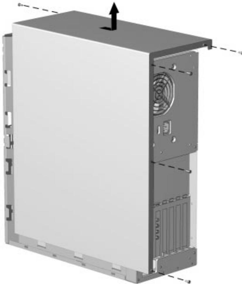
**Figure 6-5.** Removing the J Hood
