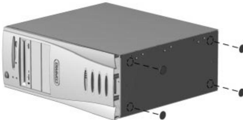
**Figure 6-2.** *Installing the Feet*
