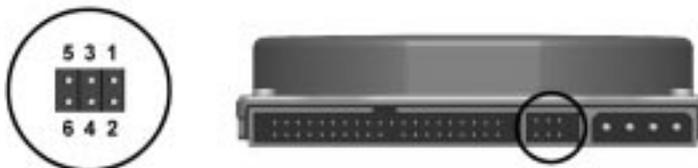
Figure 7-20. 2.4-GB Ultra ATA Hard Drive Jumper Settings
