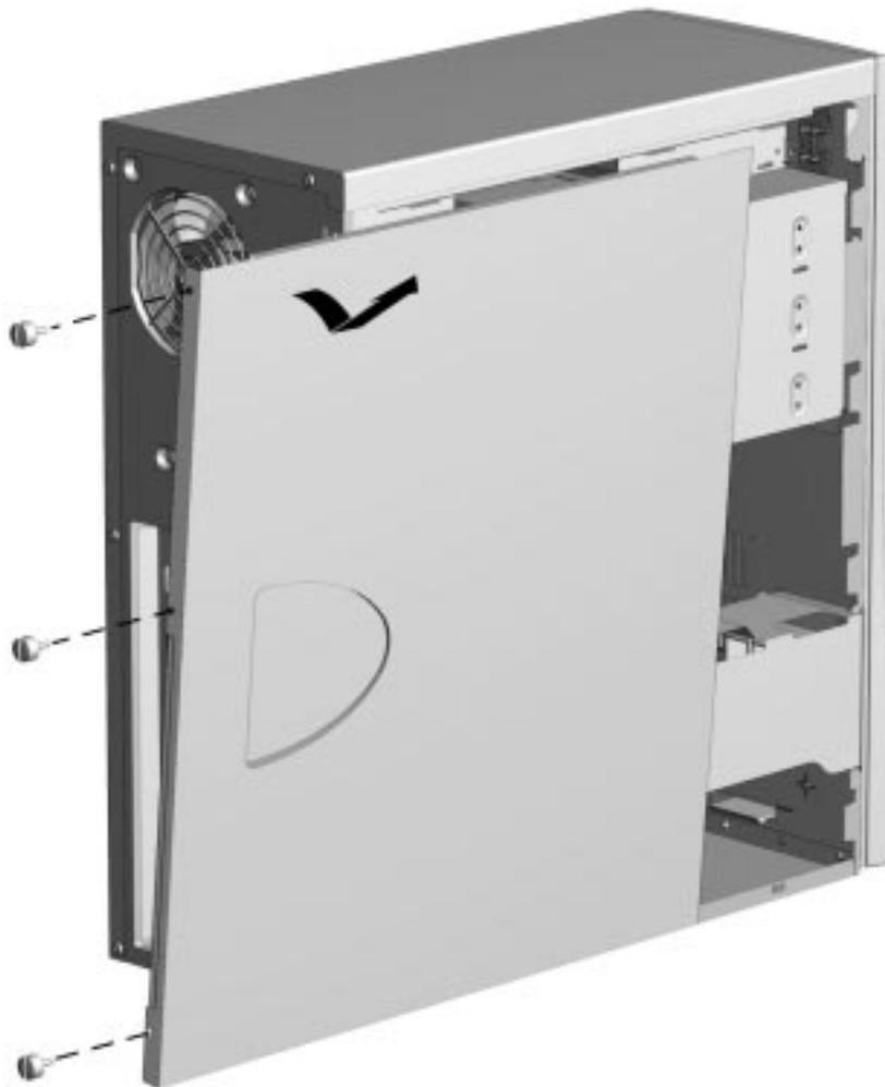
**Figure 6-4.** Removing the Access Panel
