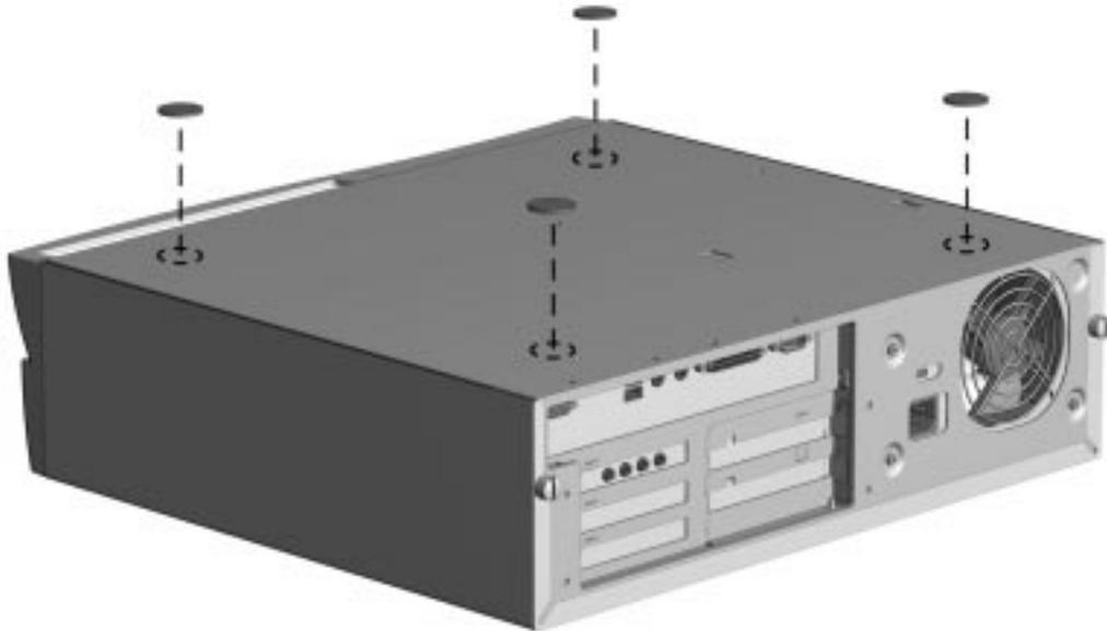
*Figure 5-2. Installing the Feet*
