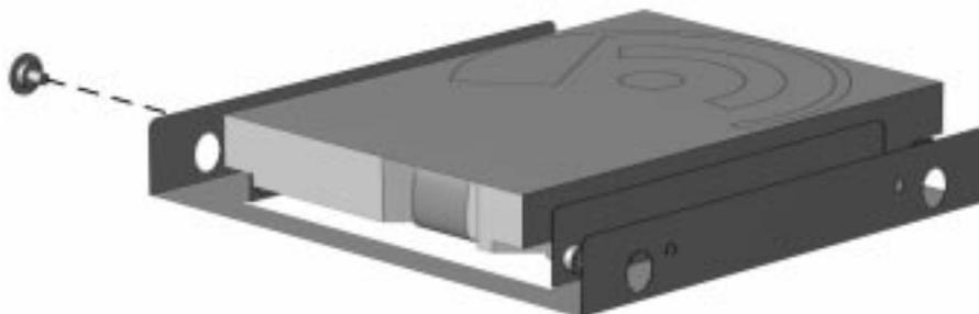
**Figure 5-34.** Inserting the Wafer Screw on the Left Side of the Bracket
