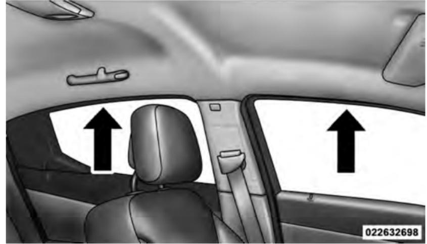
Side Airbag Inflatable Curtains (SABIC) Location
