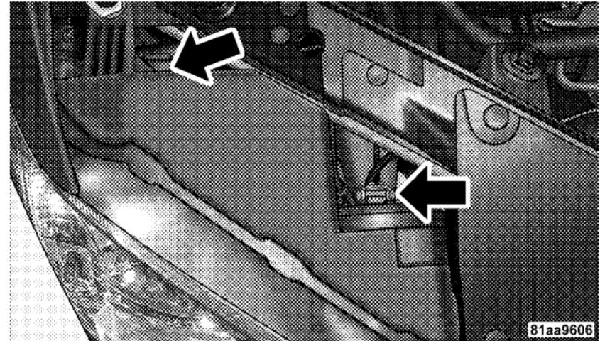
3. Rotate bulb and connector  $\frac{1}{4}$  turn and pull outward from assembly.
