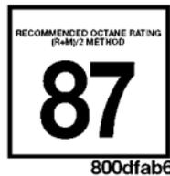
All engines are designed to meet all emission regulations and provide excellent fuel economy and performance when using high quality unleaded “regular” gasoline having an octane rating of 87. The use of premium gasoline is not recommended, as it will not provide any benefit over regular gasoline in these engines.
