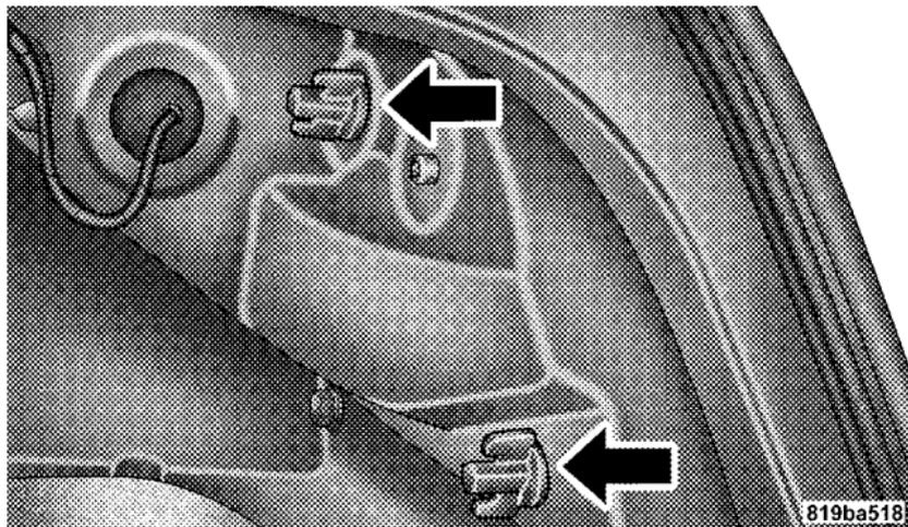
3. Grasp the taillamp and pull firmly outward pushing gently on the studs from inside to disengage the lamp housing.
