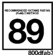
The 3.5L engine is designed to meet all emissions regulations and provide satisfactory fuel economy and performance when using high-quality unleaded gasoline having an octane range of 87 to 89. The manufacturer recommends the use of 89 octane for optimum performance. The use of premium gasoline is not recommended, as it will not provide any benefit over regular gasoline in these engines.
