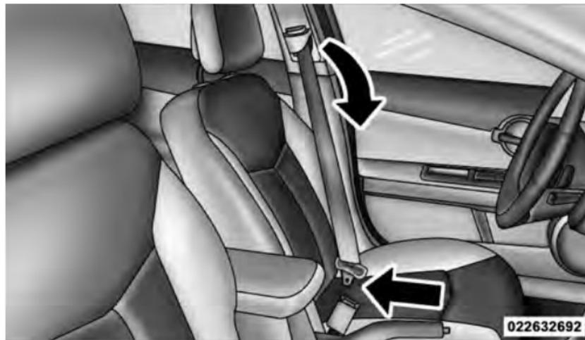
Inserting Latch Plate into Buckle
