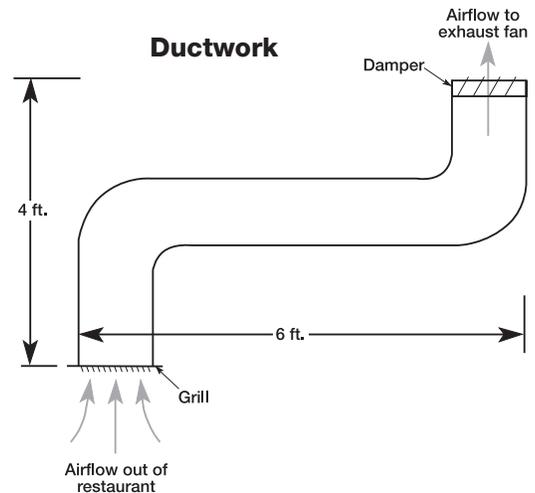
To calculate the system losses, one must know the ductwork system configuration (see Ductwork figure).
