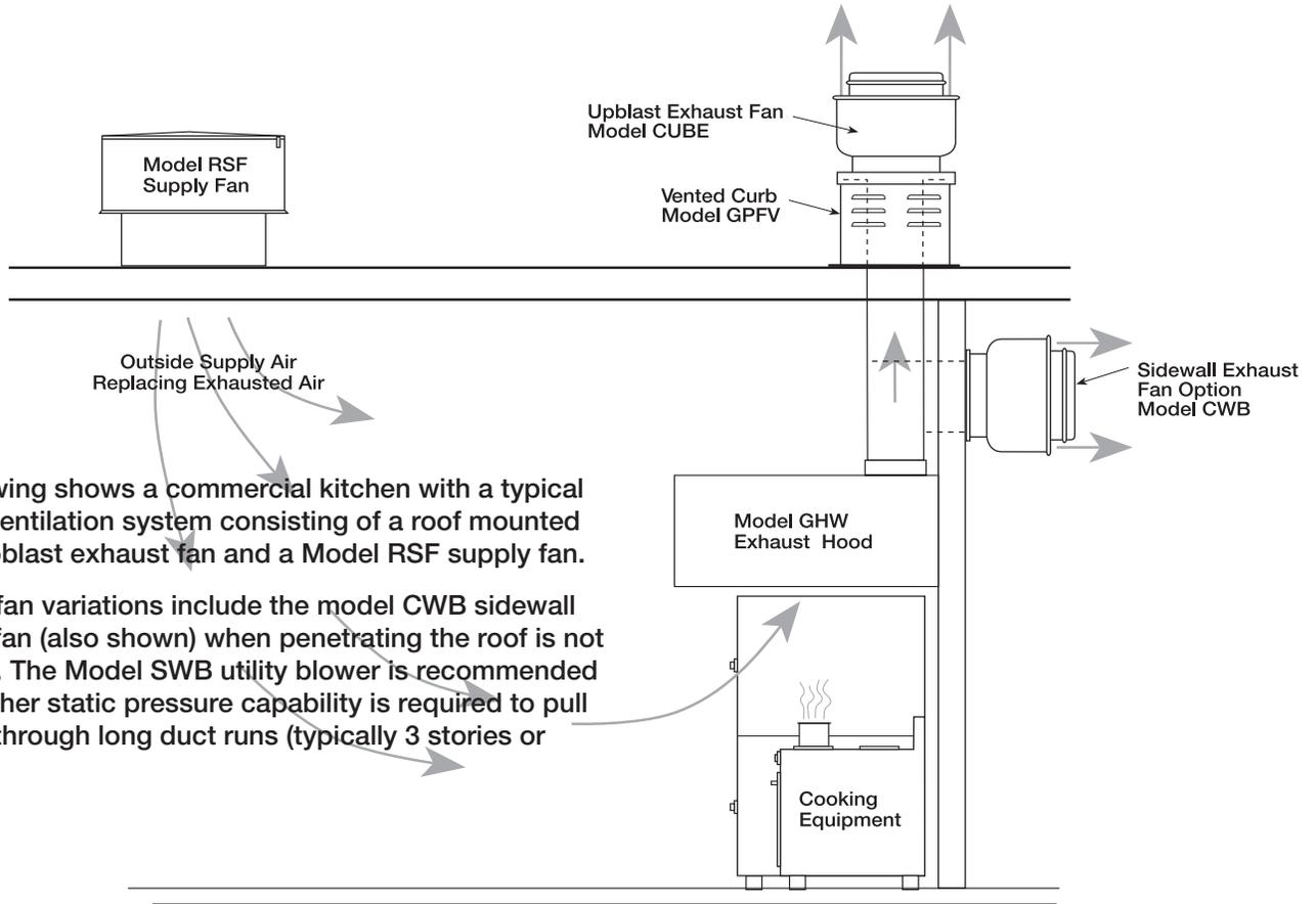
This drawing shows a commercial kitchen with a typical kitchen ventilation system consisting of a roof mounted CUBE upblast exhaust fan and a Model RSF supply fan.
