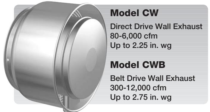
The above models are designed for exhausting relatively clean air at temperatures up to 130°F. Motors are out of the airstream. Direct drive sizes 60-95 are equipped with 3-speed motors for maximum airflow flexibility. All direct drive units except 1725 rpm (A speed) can be used with a speed control.
