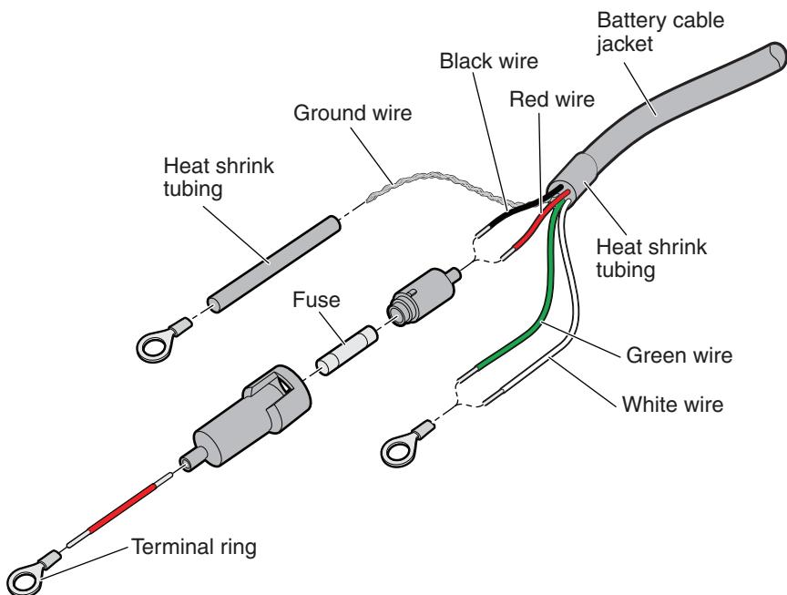
**5** Insert and secure the fuse in the fuse holder assembly.
