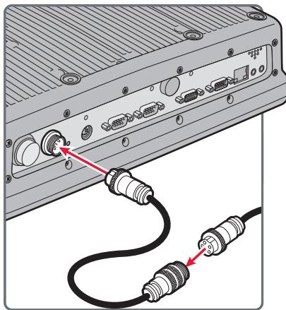
*This illustration shows connecting adapter cable P/N VE027-8024-C0 to the y-cable and a CV61.*
