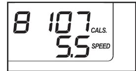
If the Start button or the Speed increase button is pressed, the walking belt will begin to move at 1 mph. As you exercise, change the speed of the walking belt as desired by pressing the Speed increase and decrease buttons. Each time you press a button, the speed setting will change by 0.1 mph; if you hold down a button, the speed setting will change in increments of 0.5 mph. Note: After you press the buttons, it may take a moment for the walking belt to reach the selected speed setting.
