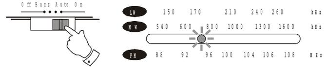
2. Select the required waveband using the **Waveband selector switch**.
