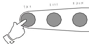
4. Whilst holding down the **Time Set button** press the **Hour**, or **Minute buttons** to set the time. Release the buttons when the correct time is reached. The clock uses a 12 hour display with a **PM indicator**. Ensure that the correct 12 hour cycle is selected.
