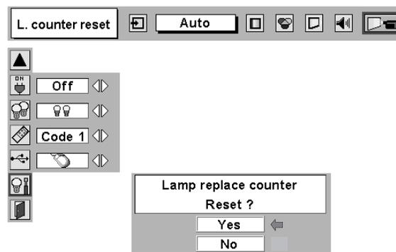
Message "Lamp replace counter Reset?" is displayed. Move pointer to [Yes] and then press SELECT button.
