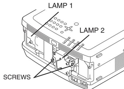
Make sure which number of lamp needs to be replaced on Lamp Status Display. Figure shows case of replacing LAMP 2.
