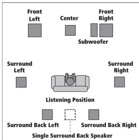
The diagrams below show suggested surround and surround back speaker orientation. The first diagram (*fig. A*) shows orientation with one surround back speaker (or none) connected. The second (*fig. B*) shows orientation with two surround back speakers connected.
