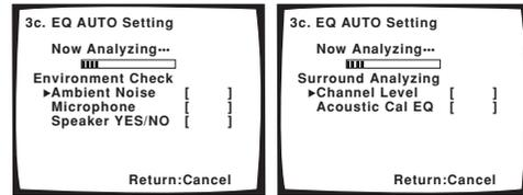
As the receiver outputs test tones, the frequency balance is adjusted automatically for the following settings:
