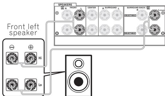
Since both front and surround back speaker terminals output the same audio, it doesn't matter which set (front or surround back) is powering which part (**Hi** or **Low**) of the speaker.
