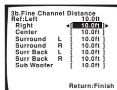
Listen to the reference speaker and use it to measure the target channel. From the listening position, face the two speakers with your arms outstretched pointing at each speaker. Try to make the two tones sound as if they are arriving simultaneously at a position slightly in front of you and between your arm span.
