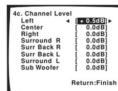
Adjust the level of each speaker as the test tone is emitted.
