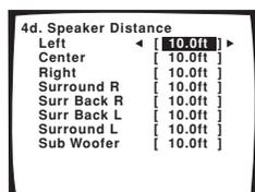
You can adjust the distance of each speaker in 0.5 feet increments.
