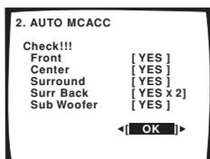
If the speaker configuration displayed isn't correct, use the **↑/↓** (cursor up/down) buttons to select the speaker and **←/→** (cursor left/right) to change the setting (and number for surround back). When you're finished, go to the next step.
