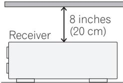
Slot and openings in the cabinet are provided for ventilation and to protect the equipment from overheating. To prevent fire hazard, do not place anything directly on top of the unit, make sure the openings are never blocked or covered with items (such as newspapers, table-cloths and curtains), and do not operate the equipment on thick carpet or a bed.
