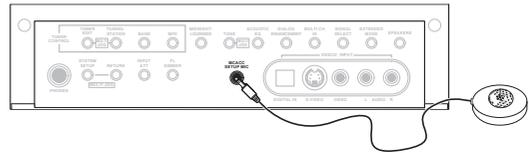
If you have a tripod, use it to place the microphone so that it's about ear level at your normal listening position. Otherwise, place the microphone at ear level using a table or a chair.
