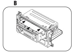
Using the alignment pins on the trim plates & the corresponding holes in the housing, attach the upper trim plate and the lower trim plate supplied with the kit.
