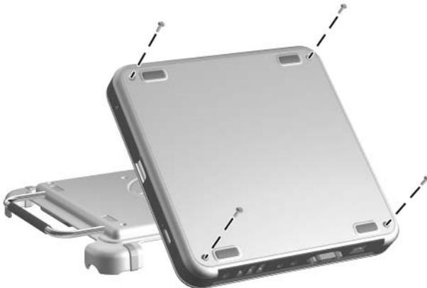
*Removing the Top Case Screws*
