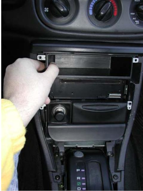
Pull the center dash rack out about 4 to 6 inches. Once you have done this, reach over to the right side and pull off the ground connector as shown in the picture on the right. Continue to pull the rack out. This step is why it is important to put the car in a gear lower than park. You will find that if you do not, you won't be able to pull the rack out. The shifter will get in your way which is very annoying when your hands are busy with other things.
