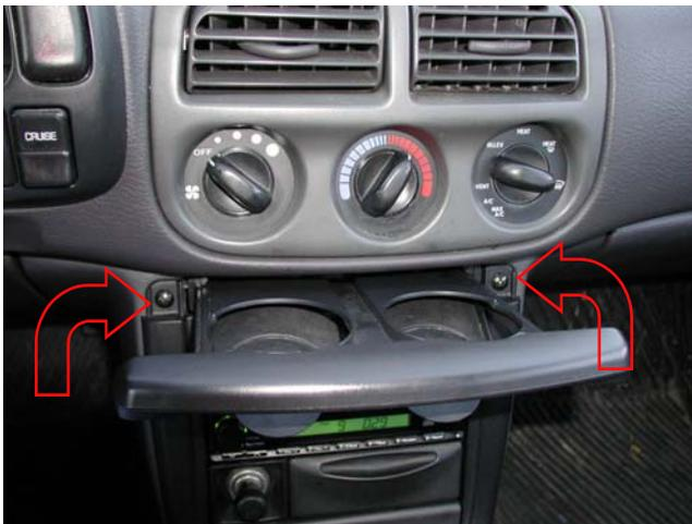
Now, open the cup holder. We are then going to remove the screws to the left and right of the cup holder. This frees the top portion of the outer trim assembly for the center of the dash.
