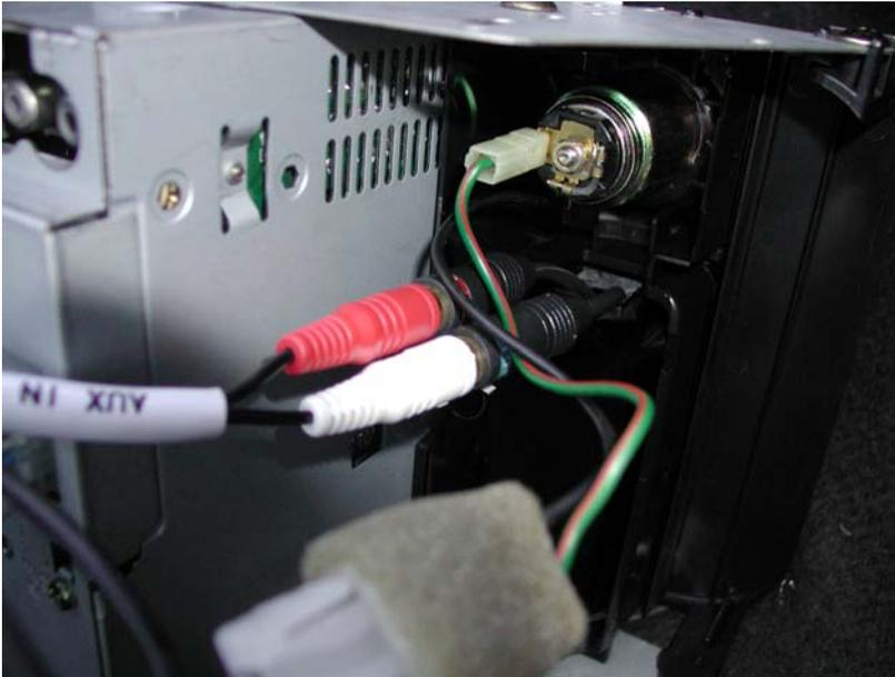
This is a picture of something else I am very happy with. I used an RCA to mini-stereo plug adapter to allow me to attach my MP3 Player to the car stereo. I wired it up to the AUX IN connector. Now when I switch to AUX IN mode I can play from a friends MP3 player or my own.
