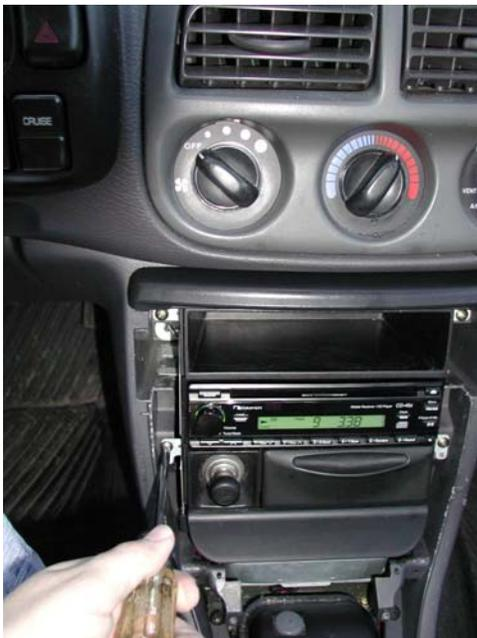
Now, remove the four screws holding in the center dash rack. This rack holds the entirely CD, ashtray, lighter, etc assembly. Be careful, underneath this unit is the airbag control system. We would not want to inadvertently damage it in the process. On the next page is a large picture showing the four screws to remove. The picture on the left is before removing them. On the right is after.
