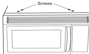
Remove 2 grille screws to remove the grill
