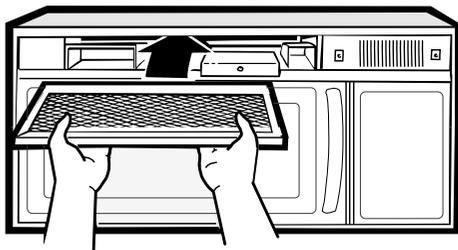
Insert the filter into the top opening of the oven as shown. It will rest at an angle on 2 side support tabs and in front of the right rear tab. Replace the grille and 2 screws.
