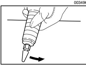
Turn the tool on without the wheel point making any contact with the workpiece and wait until the wheel point attains full speed. Then apply the wheel point to the workpiece gently. To obtain a good finish, move the tool in the leftward direction slowly.
