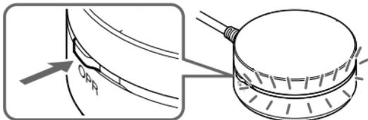
The LED status indicator starts flashing very quickly and this unit enters pairing mode.
