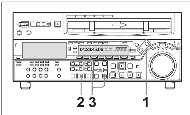
**1** When operating the player, press the **PLAYER** button, turning it on, and when operating the recorder, press the **RECORDER** button, turning it on, then stop the tapes on both the player and the recorder at the positions you wish to make the respective **IN** points.
