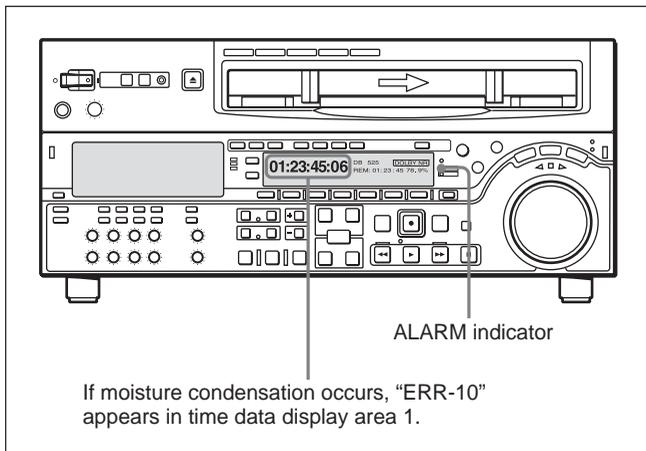
If this happens, the drum and capstan motors stop and the cassette is automatically ejected. Then, the drum starts to rotate again to dry its surface. In this state, the unit is not operable. When the moisture has evaporated, the error message disappears and the ALARM indicator goes off.
