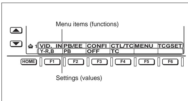
In the figure above, Y-R,B (analog component signals) is selected as the setting for VID.IN, the menu item for button F1. This manual refers to this as “F1 (VID.IN) in function menu HOME page is set to Y-R,B.”
