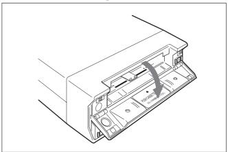
**2** After checking the tape for slack, hold the cassette so that the tape window is facing upward, then insert it into the unit.
