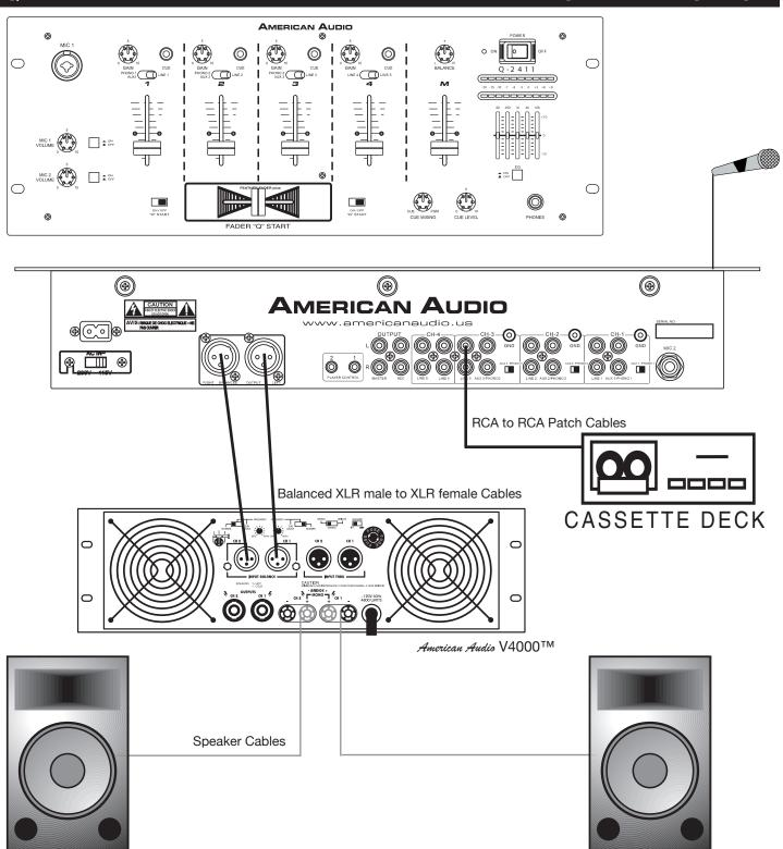
Typical Balanced Output Set-up
