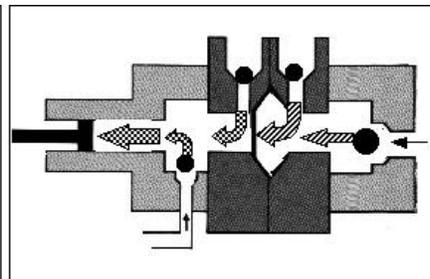
The backward movement of the piston, creates a vacuum in the hydraulic system. This causes the hydraulic outgo valve to close and the hydraulic intake valve to open (fig# 1). Opening of the hydraulic intake valve allows a new supply of hydraulic oil to enter the system, replacing the oil which was used on the forward stroke. Once again a corresponding re-action is taking place in the paint pump. The hydropulse membrane
