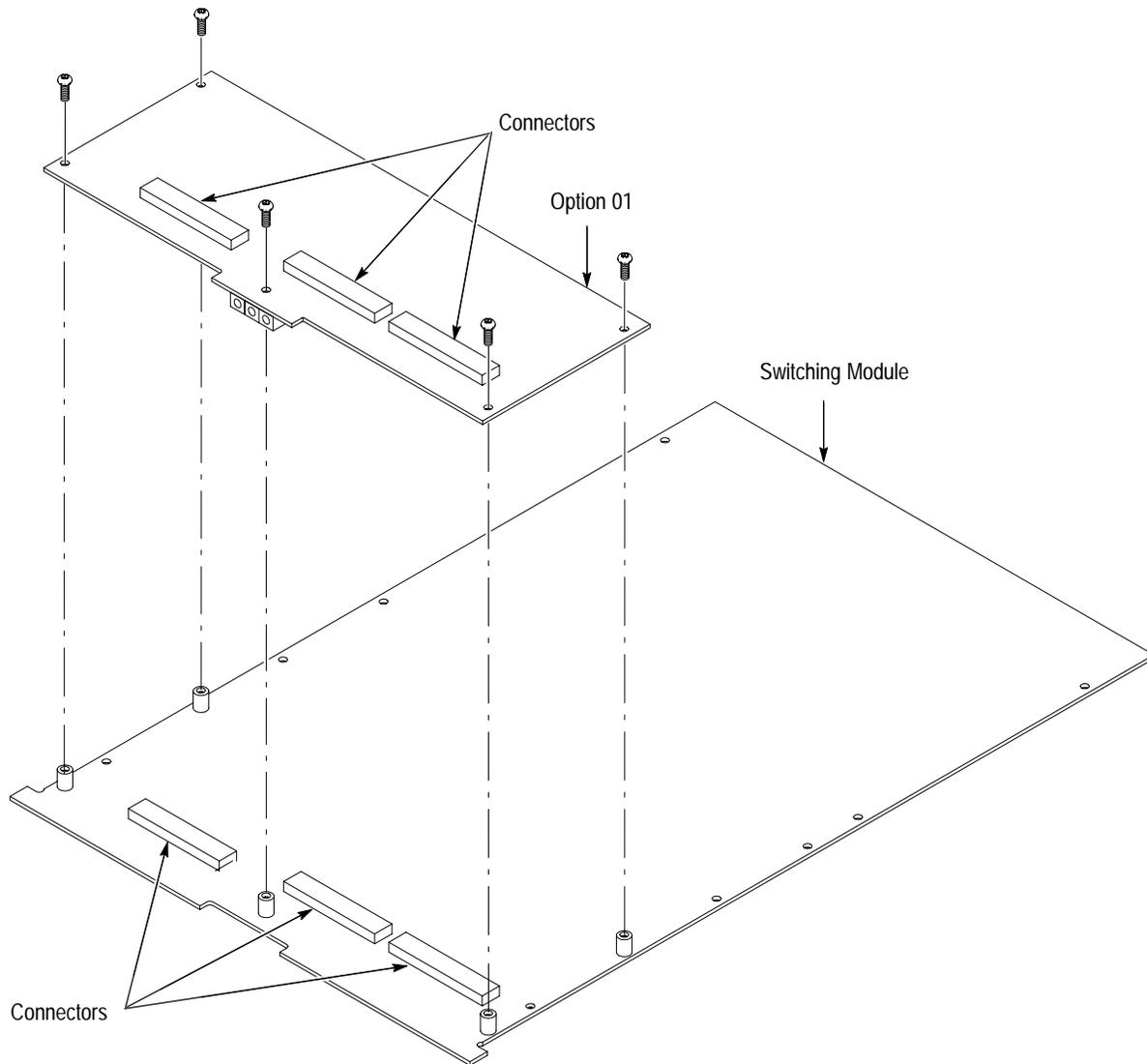
Figure 1-3: Mounting the Option 01
