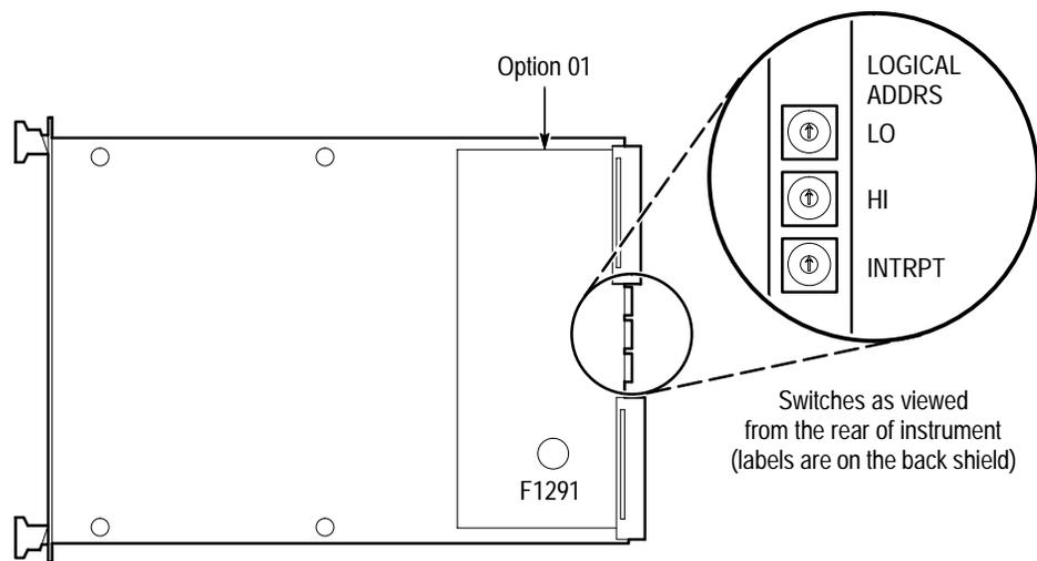
**Figure 1–1: Option 01 Indicators and Switch Locations**
