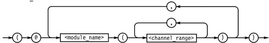
A module\_name is an ASCII string that has been associated with a relay module in a ROUTe:MODUle:DEFine command. A channel\_range may consist of a single relay number or a range of relay numbers. A range of relay numbers is indicated by two relay numbers separated by a “:” character.
