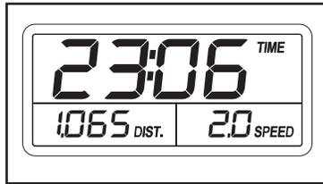
meters that you have walked or run. The lower right corner of the display can show the speed of the walking belt in kilometers per hour and the approximate number of calories you have burned.
